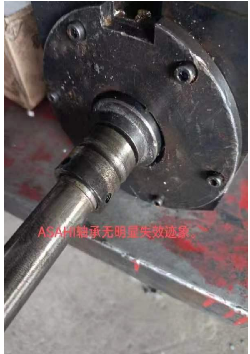
ASAHI bearing no obvious signs of failure
