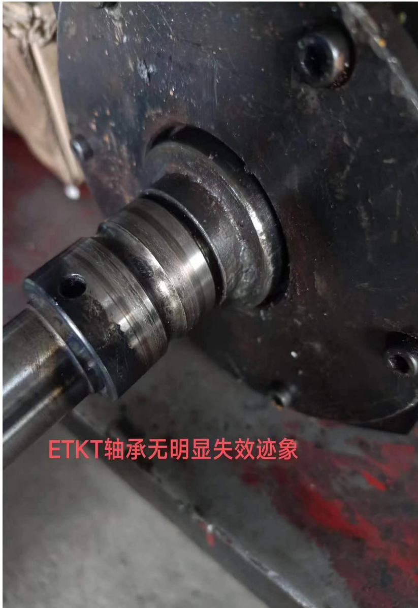
ETKT bearing no obvious signs of failure
